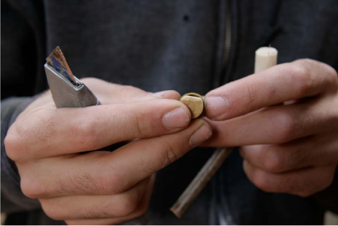
Image shows the gap created when flattening the top of the plug.
