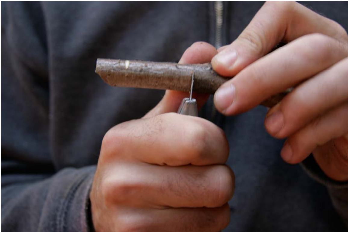
Scoring the bark so that you can slip the bark off the stick. Score all the way around the stick and through the cambium layer.
